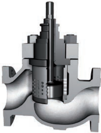
Figure 6: Mark One with CavControl Trim Body Assembly
