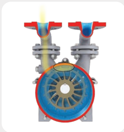
Process gases, liquids and vapors enter the compressor inlet.
