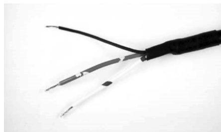
Figure 3.6 - Applying heat shrink tubing
