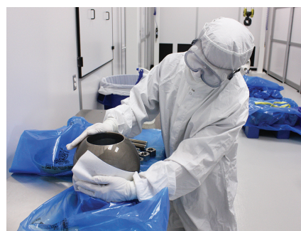
MOGAS' dedicated cleanroom prepares valves for an oxygen-enriched environment.
