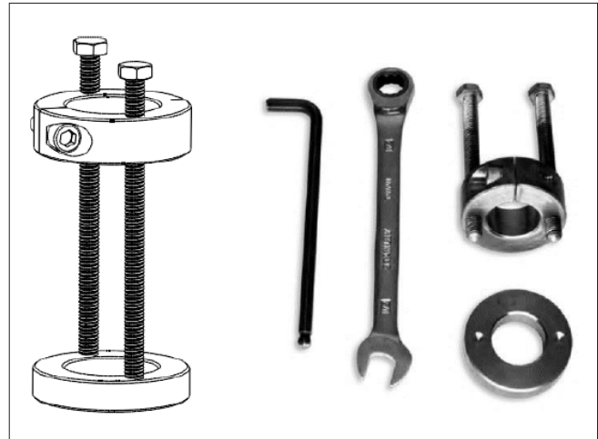
Figure 28: Shaft Removal with tools
