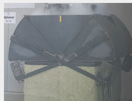
Hot oil submersion testing
