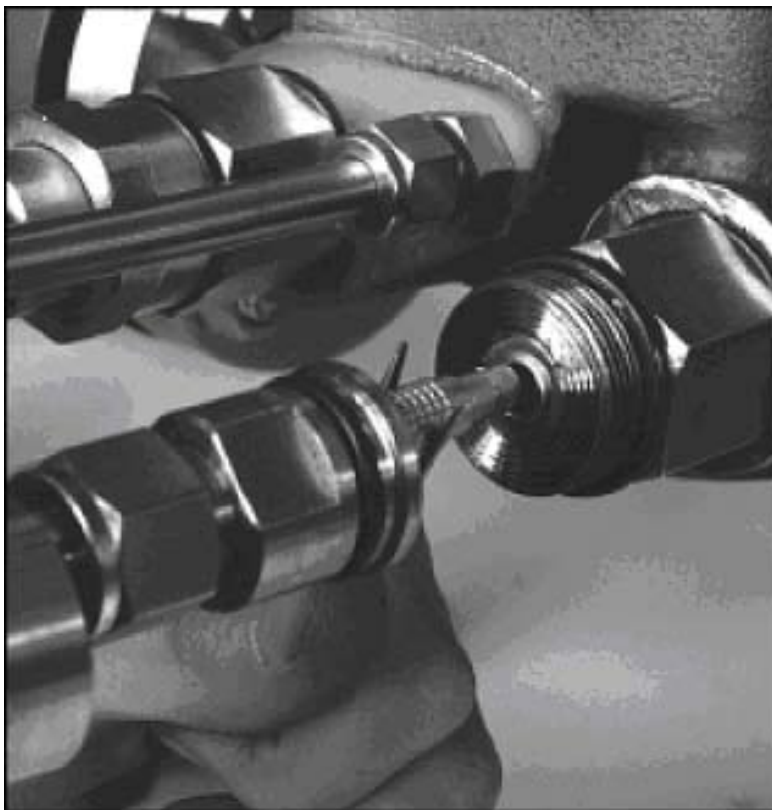
Figure 10: Disconnecting Lemo™ Connector
