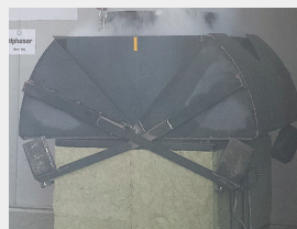
Hot oil submersion testing
