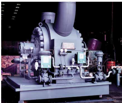
Figure 5. A radially split, forged barrel reactor feed pump for nuclear service.
