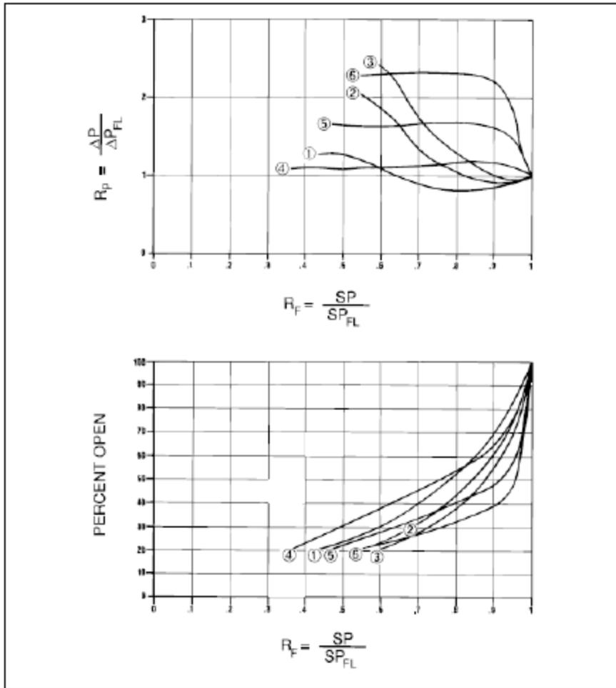
Figure 4: Edward cast steel globe and piston-lift check valve performance curves
