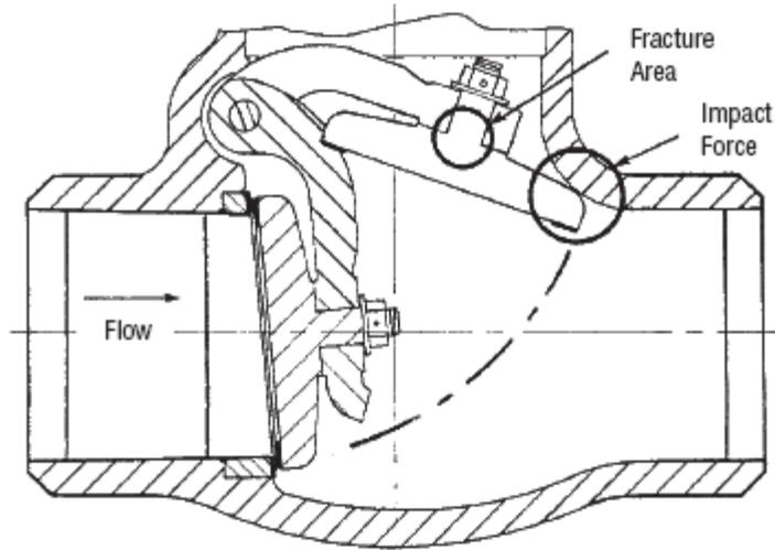
The fracturing of swing check valve disc pins has been an ongoing problem for valve manufacturers and users. The prevailing opinion is that the cause of the problem is due to disc rotation on the pin, or “turbining.”
