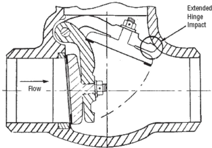
As a result of these findings, Anchor/Darling Valves modified its swing check valve design. The hinge has been extended to absorb the impact in the opening mode (Figure 2). This feature eliminates disc pin fractures while providing the disc flexibility essential to an extended seat life.
