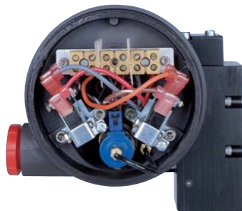
Intrinsically safe* package with SPDT gold-plated mechanical limit switches, solenoid and spool valve
